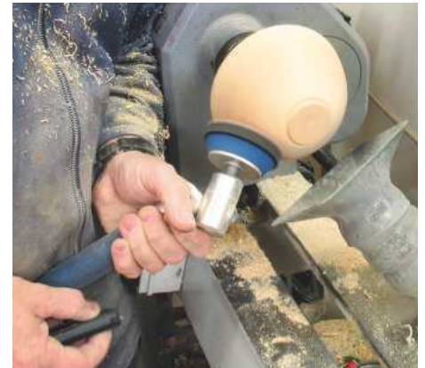
▲ Pic.3 Sanding faceplate work is always a problem as sanding marks tend to show up more than on spindle work. I'm using the Simon Hope Pro Sander, which spins as it's held against the timber
